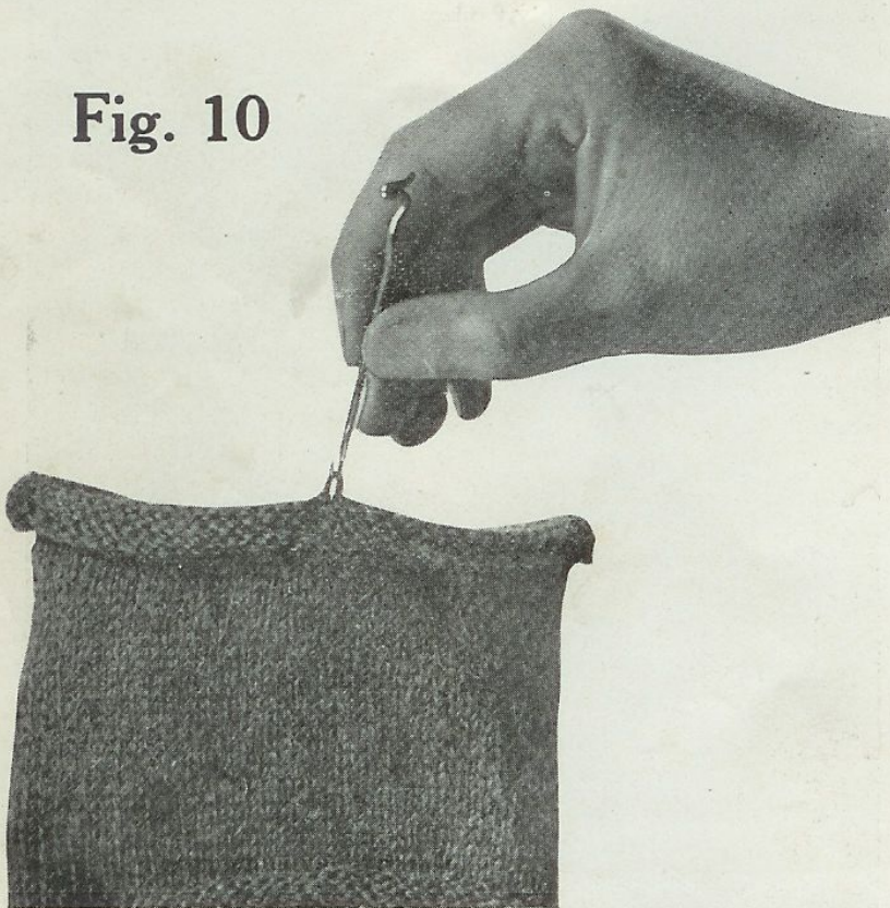
Cut showing a piece of fabric having top rolled over and how loops are pulled out to start the machine
