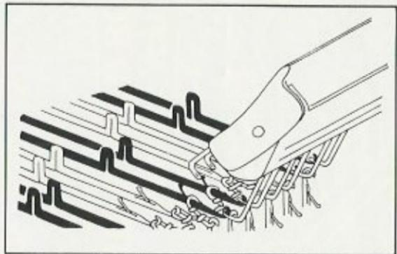
1. Arrange the required number of needles in C position that will be transferred to the Ribber.
