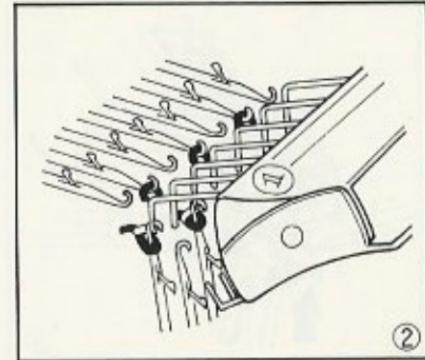
Push the Knitter needles from A to B position. Open the needle latches on both the Knitter and Ribber.
