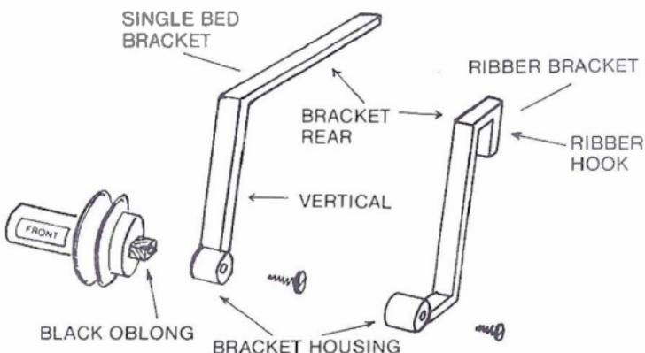
**ASSEMBLY** Select Single Bed Brackets or Ribber Brackets as appropriate. With 'FRONT' label facing towards you, place Bracket Housing on Black Oblong with Bracket Rear away from you. Insert Screw and tighten (see diagram).
