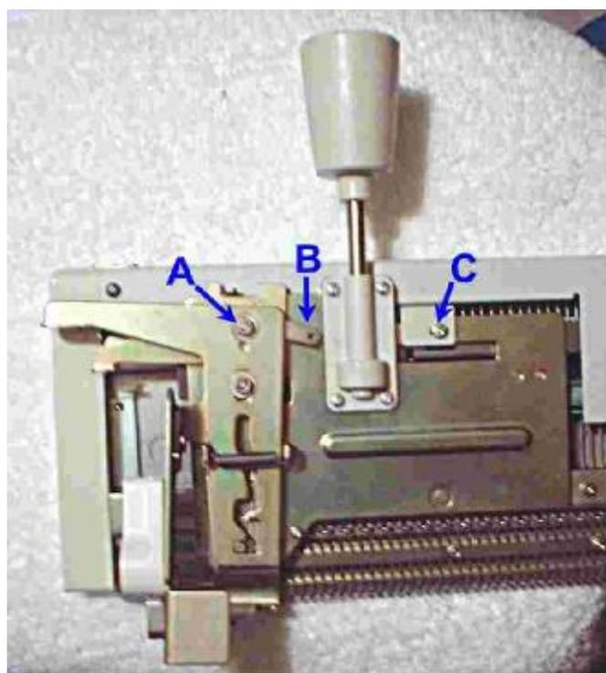
If this works tighten the screws and replace the clamps. If more adjustment is required you need to loosen the screw shown as ‘C’ beside the racking handle holder. This releases the machine bed from the racking positions and it can be moved a small distance from side to side. With the beds racked to where they should be exactly matching, at H 5 for the standard gauge, move the ribber until the needles are exactly opposite before tightening the screw.
